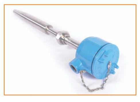
sintered Tungsten carbide Thermowell would form typically, a complete assembly for use in Power Plants for highly abrasive services such as mill classifier outlet for temperature measurement of Coal + Air mixture. For use at relatively high temperatures we recommend re-crystallized Silicon carbide, which also has very high abrasion resistance characteristics.
