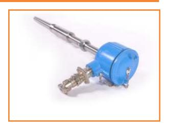
and nipple-union-nipple in 316 SS as a standard feature in weatherproof or flameproof execution. This will resist atmospheric corrosion and help in carrying out periodic maintenance with more ease. Heavy duty well with process connection of 1.5"NPT and tapered shank tapering from 38mm to 33mm is offered as a standard design for use on very high pressure application such as syngas compressor discharge.
