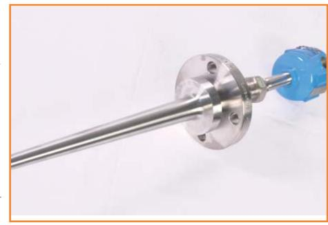
For highly corrosive services, Thermowells without a weld joint are recomended. If weld joint cannot be avoided, full penetration weld is carried out and checked by 100% radiography test. The design shown in this leaflet fulfills this criteria. Thermowells can also be offered with PWHTof weld joint, hardness check as per NACE MR-01-75, DP test, hydro test and ferrite number test.
