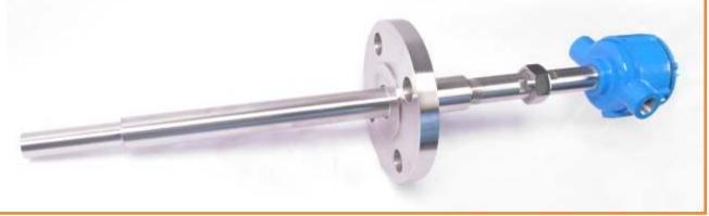
MI Thermocouple or Resistance Thermometer sensor fitted into a terminal head, and provided with head extension and drilled bar stock flanged thermowell would form a typical complete assembly ready for use in the application designed for. High velocity collar can be provided to reduce the suspended length of Thermowell and to meet ASME PTC 19.3 requirement.
