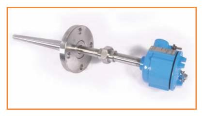
MI Thermocouple or Resistance Thermometer sensor fitted into a terminal head, and provided with head extension and drilled bar stock flanged thermowell as per ENI standard 0165.00, is ideally suited for use in Fertiliser plants, Refineries and Petrochemical complexes.
