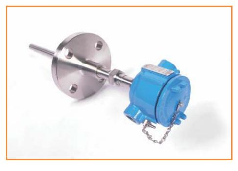
depends on various process parameters, such as, temperature, dynamic pressure, flow velocity, abrasive nature of process fluid, intricate nature of installation and insertion lengths required. High velocity collar can be provided to reduce the suspended length of Thermowell and to meet ASME PTC 19.3 requirement.
